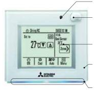
Brightness sensor: If room light is on, energy-saving control is deactivated.
