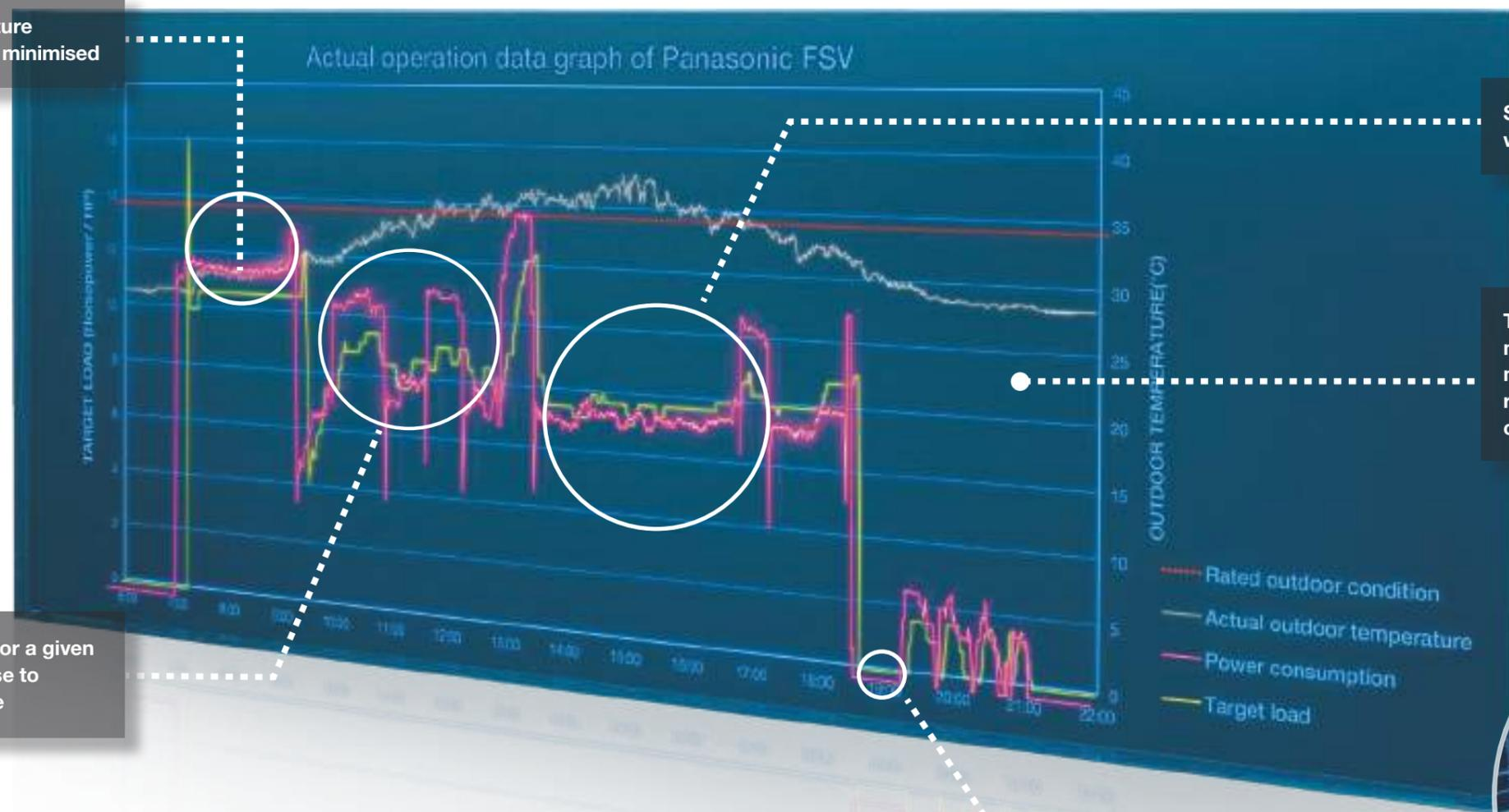
Set temperature maintained with minimum load operation
